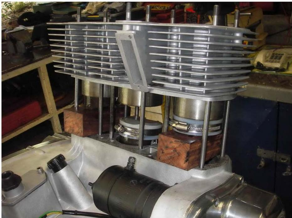
Remove two outer Nylon strips and Hose clamps, rotate engine carefully so middle piston comes up towards TDC but stop before outer pistons reach the oil rings, you will have room below the middle piston to insert 2 x 3/16" strips of steel in under the side of the skirts in line with the Gudgeon Pins, line piston up, strike barrel with hands again, will slide straight down, remove hose clamp and nylon strip.
