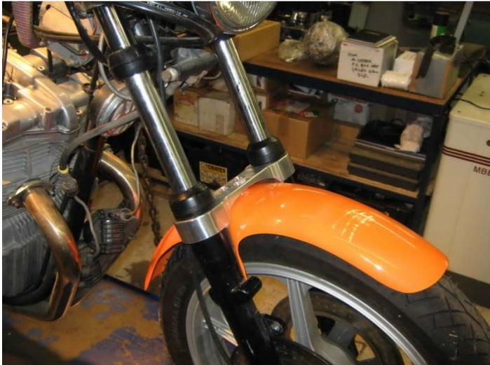
*Fork Brace shown at left mounted onto a Monty. Brace is not one of the Tarozzi units as mentioned in this article.*
