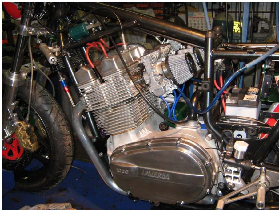
Photo shows a highly modified 77 triple with the Dyna green coils mounted in place.
