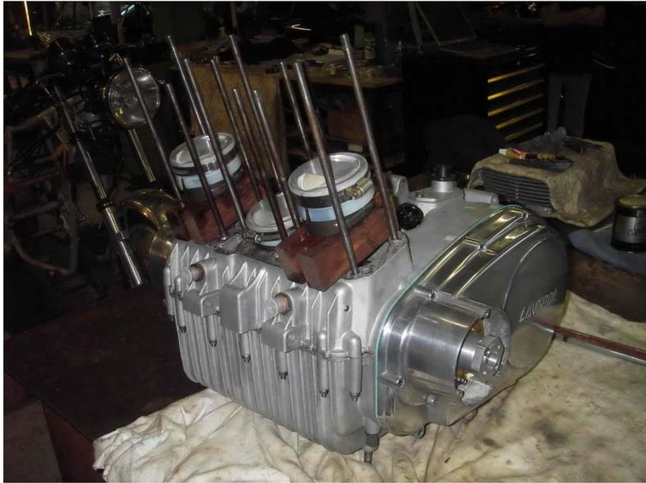
Quick, simple, cheap, ring compressors shown above. Three strips of Nylon cut to length to wrap around the pistons neatly. Make them approx 25mm wide, thickness is around 2-3mm. Three suitable hose clamps, tighten clamps up as tight as possible then back off 1 turn, should be able to turn the nylon strip and hose clamp on the Piston. Hose clamps should be at the top of the strip, approx 2 mm from the top and even all around.
